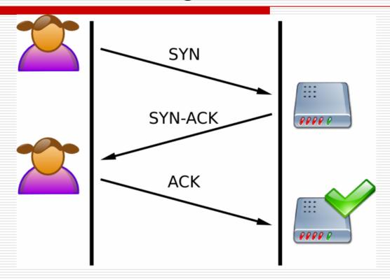
A normal connection between a user and a server. The three-way handshake is correctly performed.
